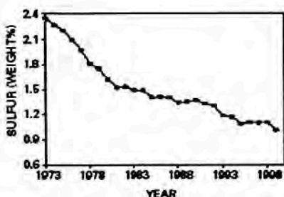
Figure 2. Sulfur content of coals used at U.S. powerplants, 1973 to 1999. Data from the Federal Energy Regulatory Commission (available at http://www.ferc.fed.us/electric/f423/f423annual.htm ).
